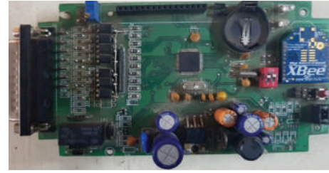
FIGURE 5: Hardware of PIC16f877a with Zigbee.
