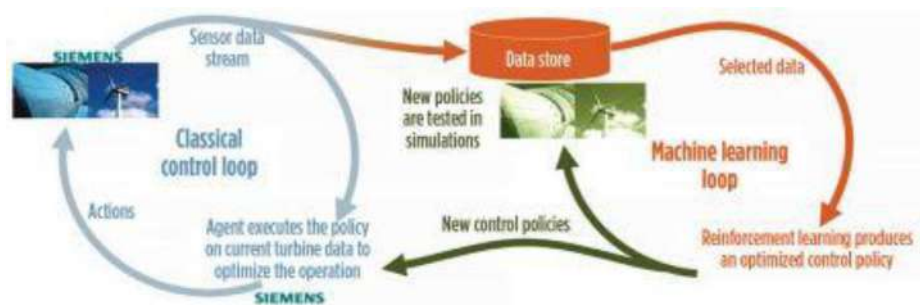
Fig. 3. Automation Control Loop with Machine Learning.
